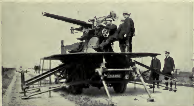
No. 2.—3-inch 20-cwt. Q.F. high-velocity gun on high-angle anti-aircraft mounting and Daimler chassis.
